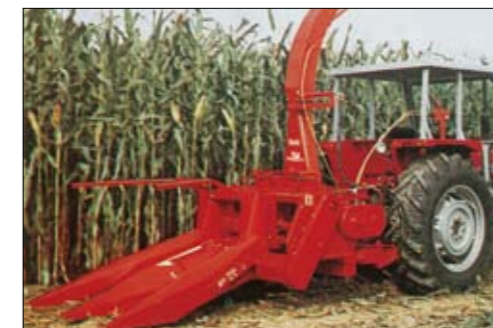
Forage harvester 946 with 2 row maize head Model 21 for chopping complete maize plants, planted at 60 to 80 cm row spacing
