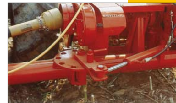
Patented hydraulic re-positioning system from rear to side of tractor mounting
