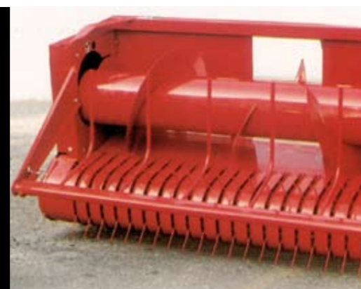
Pick-up with feeding auger
