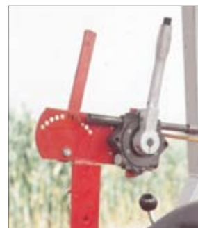
Remote control for spout and deflector and for overload protection.
