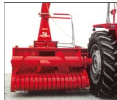
Forage Harvester Model 946 with pick-up model 50 with auger for chopping green silage which has already been cut and windrowed
