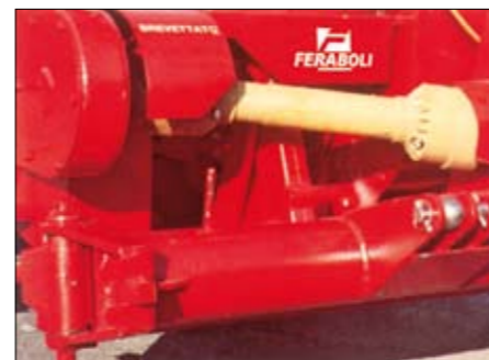
Articulated joint to change from reverse to forward drive side-mounted position and vice versa
